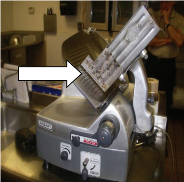
Meat scraps can accumulate under the handle of the slicer due to gaps in the silicone pieces. The meat scraps could then degrade and leach onto food being sliced.
